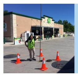
Stick tanks periodically to check the accuracy of automatic tank gauge readings. Stick checking after a heavy rain or receiving a load of fuel should be company policy.
