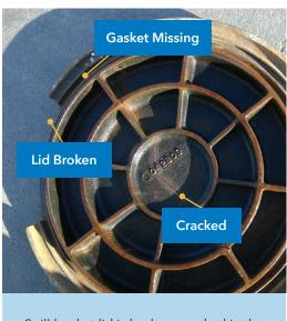
Spill bucket lid is broken, cracked in the middle and missing a rubber gasket.
